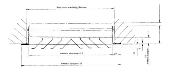
F.N.W. Type CD Ceiling Diffusers have fixed non- ñ adjustable louvres at 40mm centres. Manufactured in zinc coated steel, spot-welded construction and polyester powder coated after manufacture. A self-coloured plastic extruded flange facing being fitted over the steel flange to finish.
