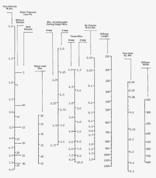
Assuming that the Air Volume and Forward Throw (either 4-way or 2-way) are the known factors, then from the above nomogram, place a rule intersecting these factors, read off Face Velocity, Static Pressure Loss, Noise Level and the Free Area of diffuser to fulfill those conditions. Pivoting the rule about the Free Area determined, the Diffuser Length and Width can be read off.
