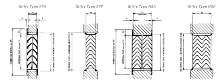
TYPE ATA plastic faced - steel air transfer grille is supplied in two halves each being flange fixed to either side of the opening and each being constructed with fixed louvres at an inclination of 45 at 25mm centres.
